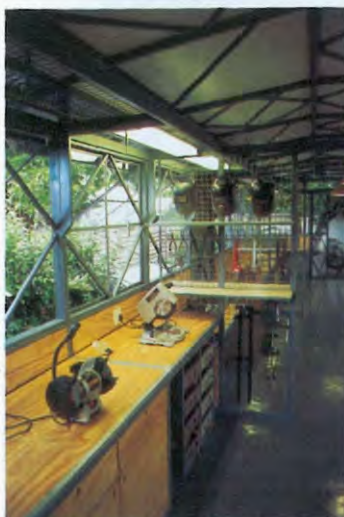
Above: Weld-mesh racking provides for further storage where everything stored can be seen. Discarded ammunition cases are used in the drawer units.
